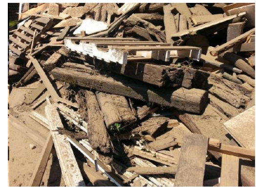
Class A IV - hazardous waste
